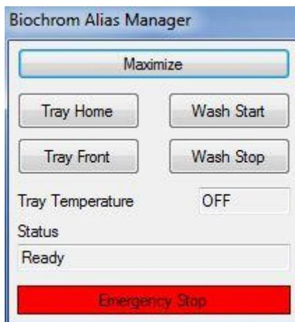
This window is triggered when the minimize button is clicked on the main Alias Manager window. It contains all the basic information along with main operations buttons. To recover the full window of the Alias Manager, click on **Maximize**.
